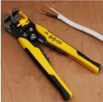
Self-adjusting wire stripper
