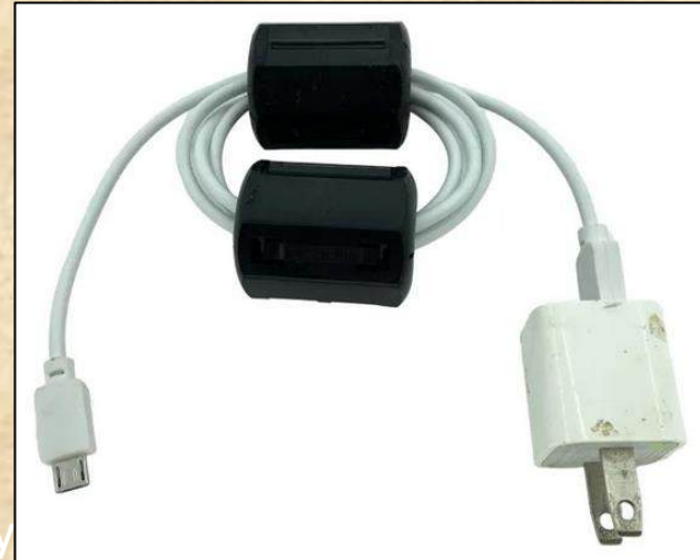
Multiple ferrite beads and loops – You are only limited to the amount of beads you can install on the loop
