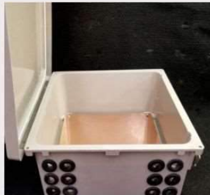
Copper sheet is easily removed by unscrewing four stainless nuts.
