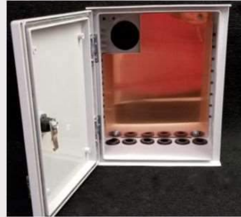
This small box (12"x10"x6") is set up as a wall mounted entry panel. 6 grommet holes bottom for cables entering box, and a cut out for 1.5" conduit in the back upper left corner for cables exiting the box.
